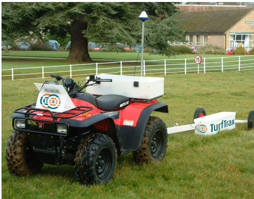
Soil scanner – 'the buggy'
